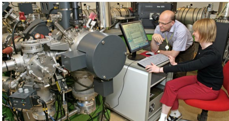
Researchers, primarily from the Nordic countries, use the ion microprobe at the NORDSIM laboratory to carry out isotope analysis at a microscopic scale.
